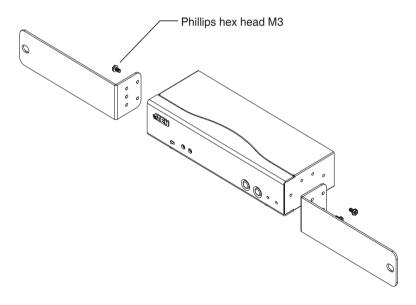
2. Screw the bracket into any convenient location on the rack.
